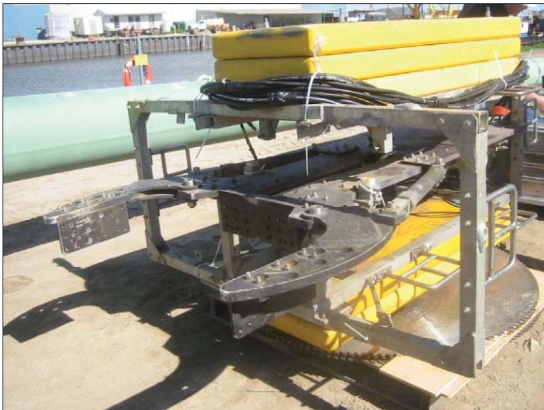
An ROV would fly this saw to pipe locations needing cutting, attach it, and leave it behind to be operated by the ROV pilot. The 60-in. diameter carbide-tipped blades shown below the tool would be attached prior to deployment (Fig. 6, photo by Christopher E. Smith).
